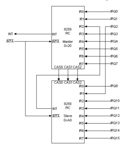
The CPU only has one interrupt line, thus the second controller had to be connected to the first controller, in a master/slave configuration. IRQ2 was selected for this. By using IRQ2 for the second controller, no other devices could use IRQ2, so what happened to all these devices using IRQ2? Nothing, the interrupt request line found on the bus, was simply diverted into the IRQ 9 input. As no devices yet used the second PIC or IRQ9, this could be done.
