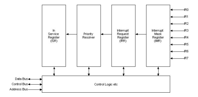
The basic block diagram of the PIC is shown above. The 8 individual interrupt request lines are first passed through the Interrupt Mask Register (IMR) to see if they have been masked or not. If they are masked, then the request isn't processed any further. However if they are not masked, they will register their request with the Interrupt Request Register (IRR).
