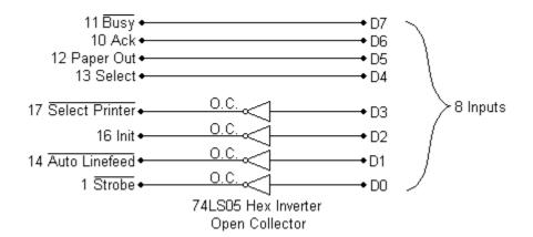
The inputs to the Parallel Port has be chosen as such, to make life easier for us. Busy just happens to be the MSB (Bit 7) of the Status Port, then in ascending order comes Ack, Paper Out and Select, making up the most significant nibble of the Control Port. The Bars are used to represent which inputs are Hardware inverted, i.e. +5v will read 0 from the register, while GND will read 1. The Status Port only has one inverted input.
