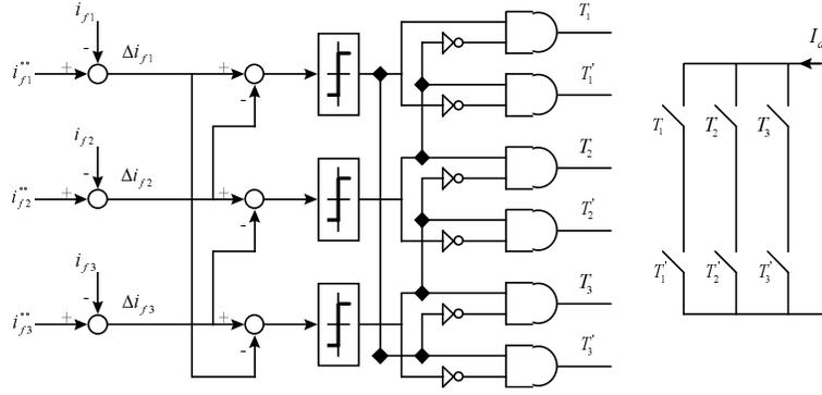
Fig. 6. Switching control of CSAF.
