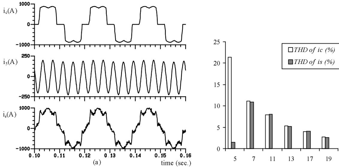
**Fig. 7.** Simulation results for 5<sup>th</sup> harmonic elimination with VSAF.
