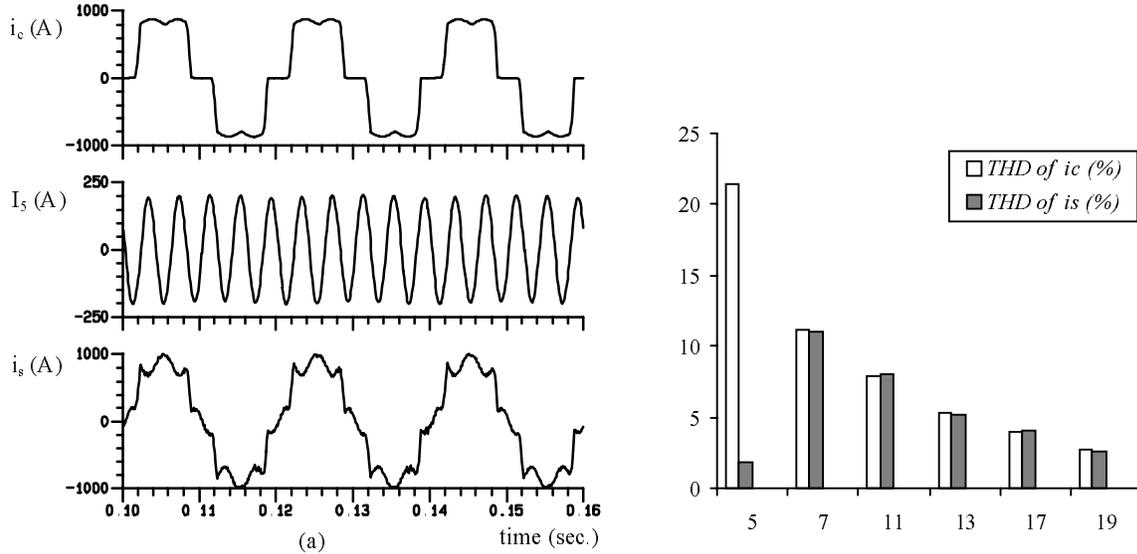
Fig. 9. Simulation results for 5<sup>th</sup> harmonic elimination with CSAF.
