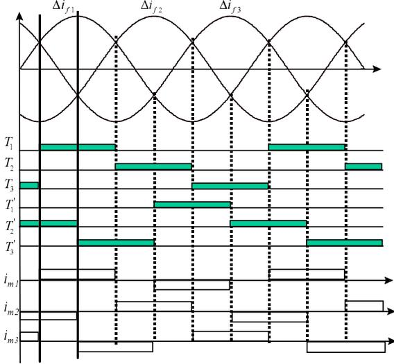
Fig. 5. The principle of the current control of CSAF.
