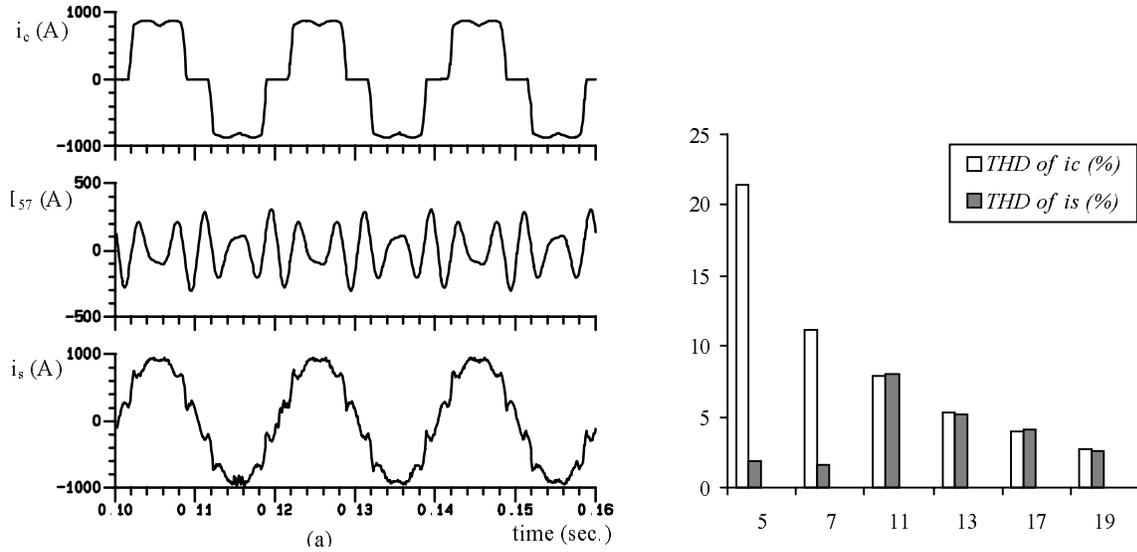
Fig. 10. Simulation results for 5<sup>th</sup> and 7<sup>th</sup> harmonic elimination with CSAF.
