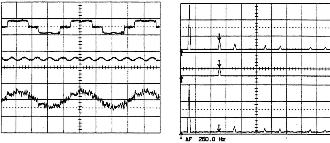
**Fig. 13.** Experimental results of elimination of the 5<sup>th</sup> harmonic, current: 25 A/div, time: 10 ms/div (from top to bottom: load current, active filter current, source current).
