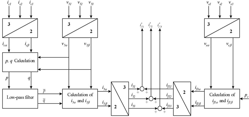
Fig. 2. Reference current calculation scheme.
