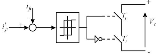
Fig. 4. Switching control of VSAF.
