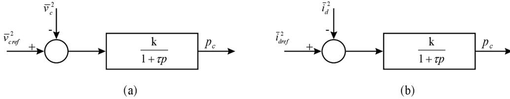
Fig. 3. Scheme of DC power control: (a) case of VSAF, (b) case of CSAF.
