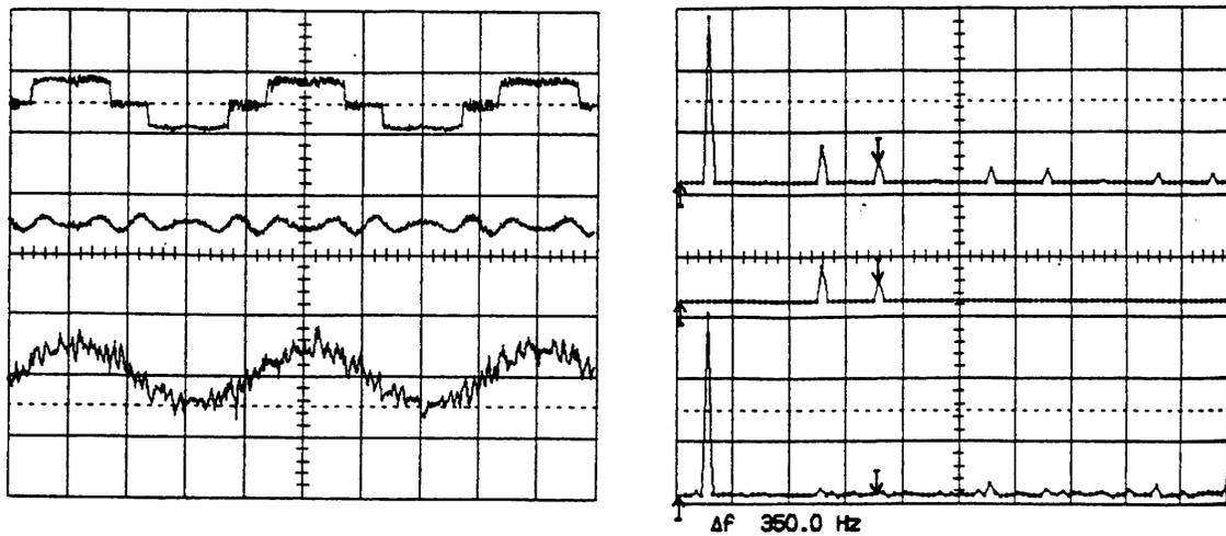
**Fig. 14.** Experimental results of elimination of the 5<sup>th</sup> and 7<sup>th</sup> harmonic, current: 25 A/div, time: 10 ms/div (from top to bottom: load current, active filter current, source current).
