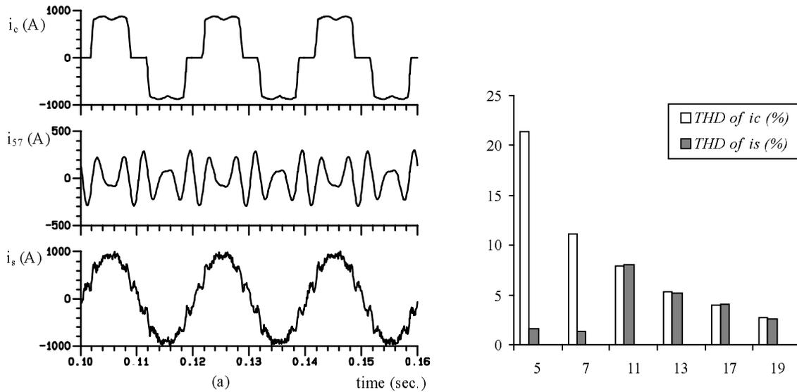
**Fig. 8.** Simulation results for 5<sup>th</sup> and 7<sup>th</sup> harmonic elimination with VSAF.
