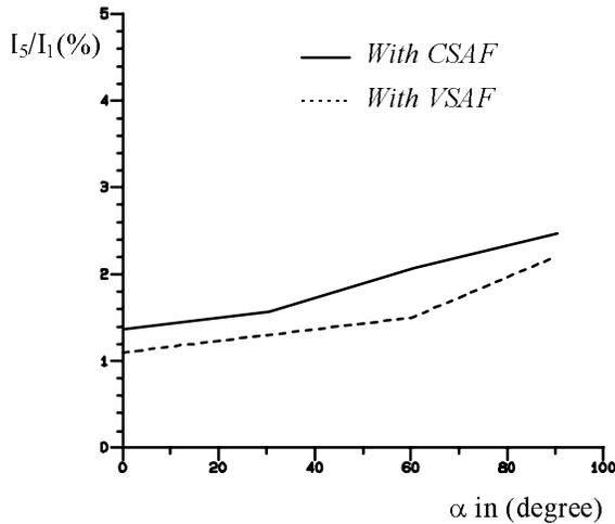
**Fig. 11.** Evolution of the 5<sup>th</sup> harmonic filtering *versus* firing angle  $\alpha$ .
