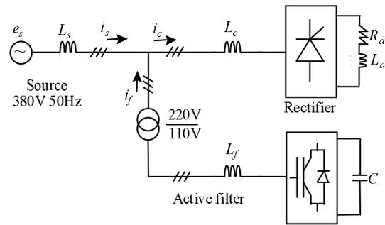
**Fig. 12.** Diagram of the experimental prototype.
