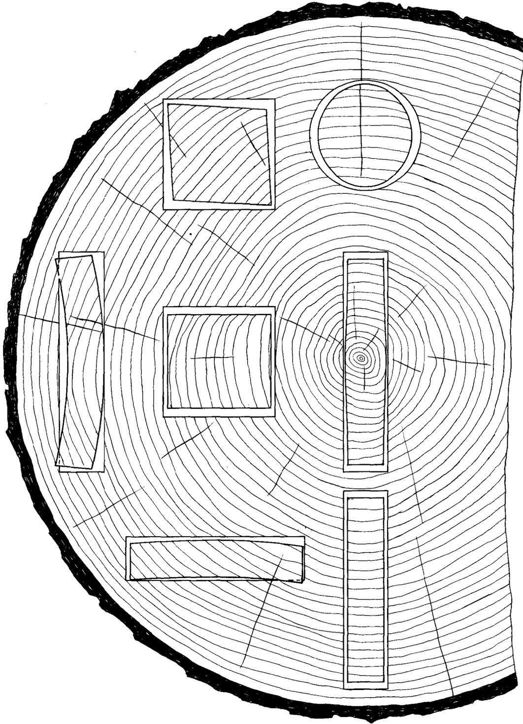
Figure 1.--Characteristic shrinkage and distortion of flats, squares, and rounds as affected by the direction of the annual rings. Tangential shrinkage is about twice as great as radial shrinkage.
